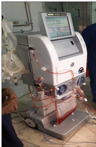
Figure 3: Performer HT specialized machine for HIPEC with its inlet/outlet tubings and chemotherapy bag.
